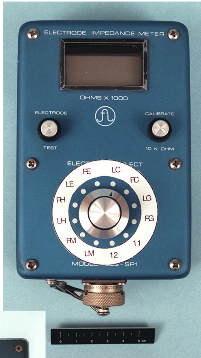
S96-18951 Figure HLS-124 Electro Impedance Meter Front View
