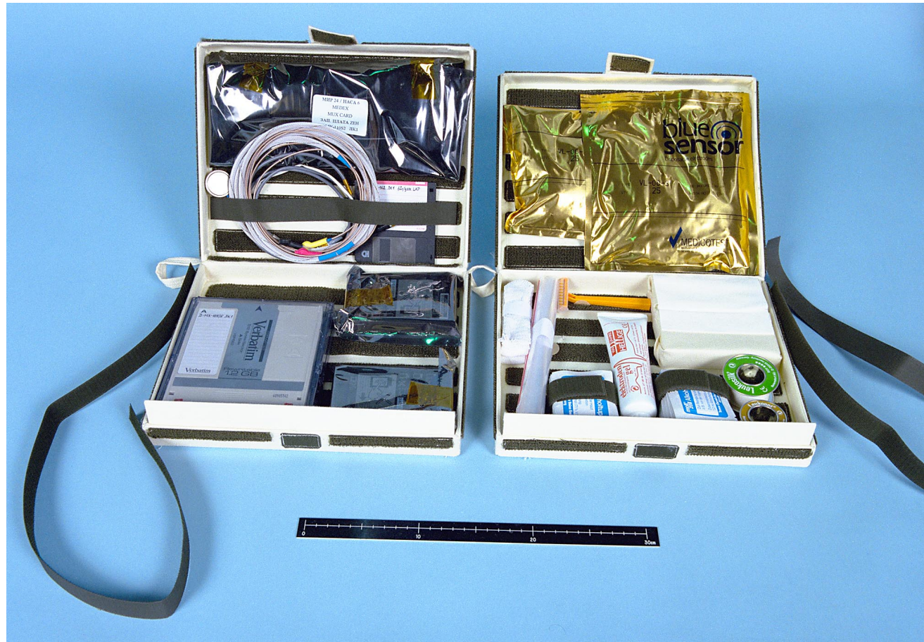
Figure HLS-50 Contents of the MEDEX Upgrade Kit (Left) and the MEDEX Consumables Kit (Right)
