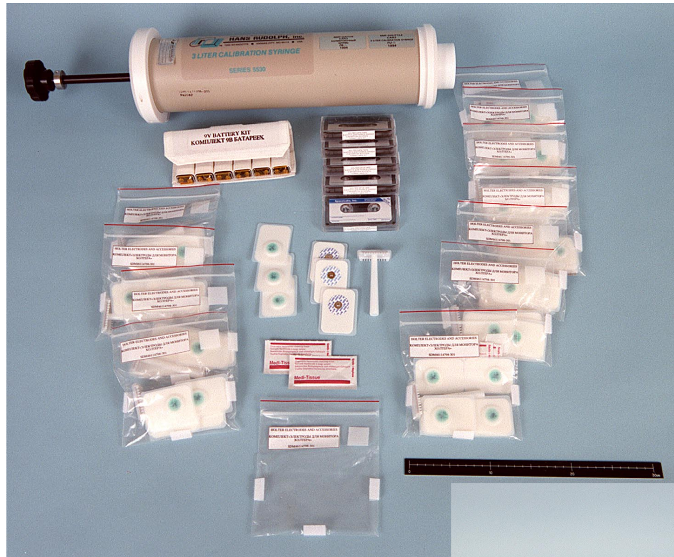
S97-10590 Figure HLS-23 Cardio Hardware: 3L Calibration Syringe, Data Tapes, and Electrodes Kit
